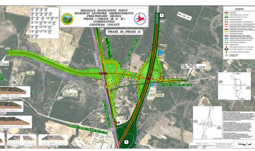
To ease access to the planned VinFast electric vehicle plant in Chatham County, the N.C. Department of Transportation wants to replace Exit 84 from U.S. 1 (bottom center) with a new interchange at New Elam Church Road, which would be relocated and extended over old U.S. 1 into the site (left). *NCDOT*
