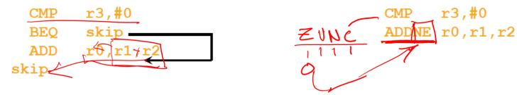
By default, data processing instructions do not affect the condition code flags but the flags can be optionally set by using <u>"S"</u>. CMP does not need "S".
